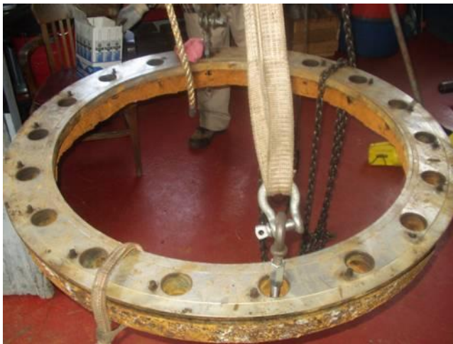
PHOTO 5 LOWER CURB RING
